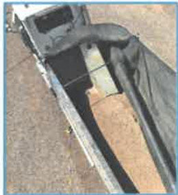
A truck driver fell 9 ½ feet while adjusting the tarp. He had climbed up the side of the truck into the bed and fell while walking on loose sand.
